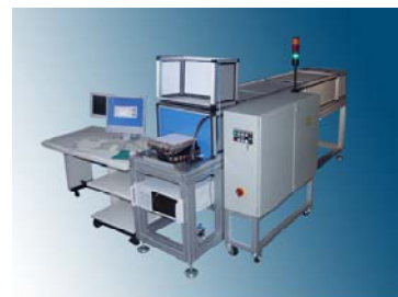
Fig. 2 Peptide laser printer
